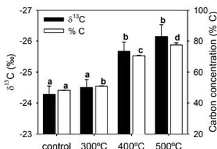
Fig. 2. Mean values and standard error for the  $\delta^{13}\text{C}$  and %C in intact wood (control) and after carbonization at a range of temperatures. Means with the same letter did not differ significantly on the basis of a least significant difference test ( $P<0.05$ ).
