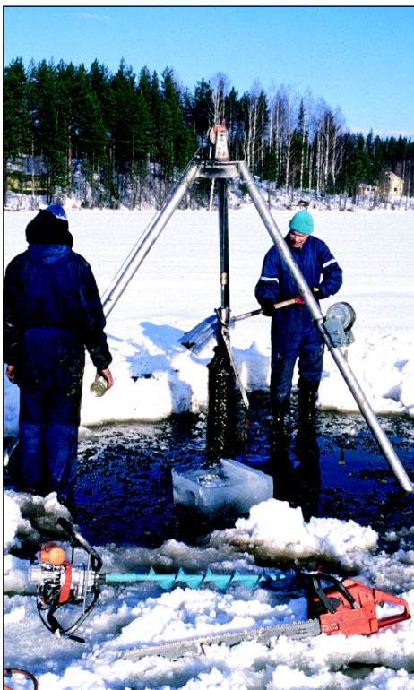
Figure 1: Kullenberg piston corer in operation on lake Pohjajärvi, Finland. The system, designed by the Geological Survey of Finland, can recover a 10 m long core in a single operation with the aid of just two people.
