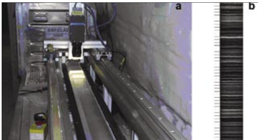
Fig. 2: As an example of the high-resolution data along the NGRIP ice core, data from the visual stratigraphy using the line scan instrument (a) is shown. A 50 cm long section of the record is shown in (b). The record is from 2358.0-2358.5 m where the age is 57 kyr b2k and the mean annual thickness is 1.2 cm.
