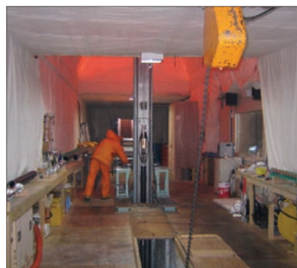
Fig. 2: Deep ice core drilling at Dome Fuji using a newly developed drill with highly efficient performance.
