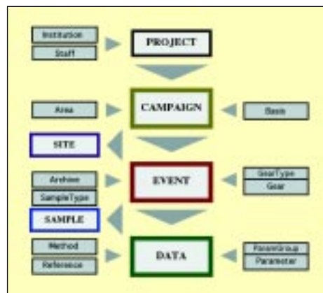
Figure 1: The hierarchy in the PANGAEA data model mirrors the path from the sampling in projects to the published data.
