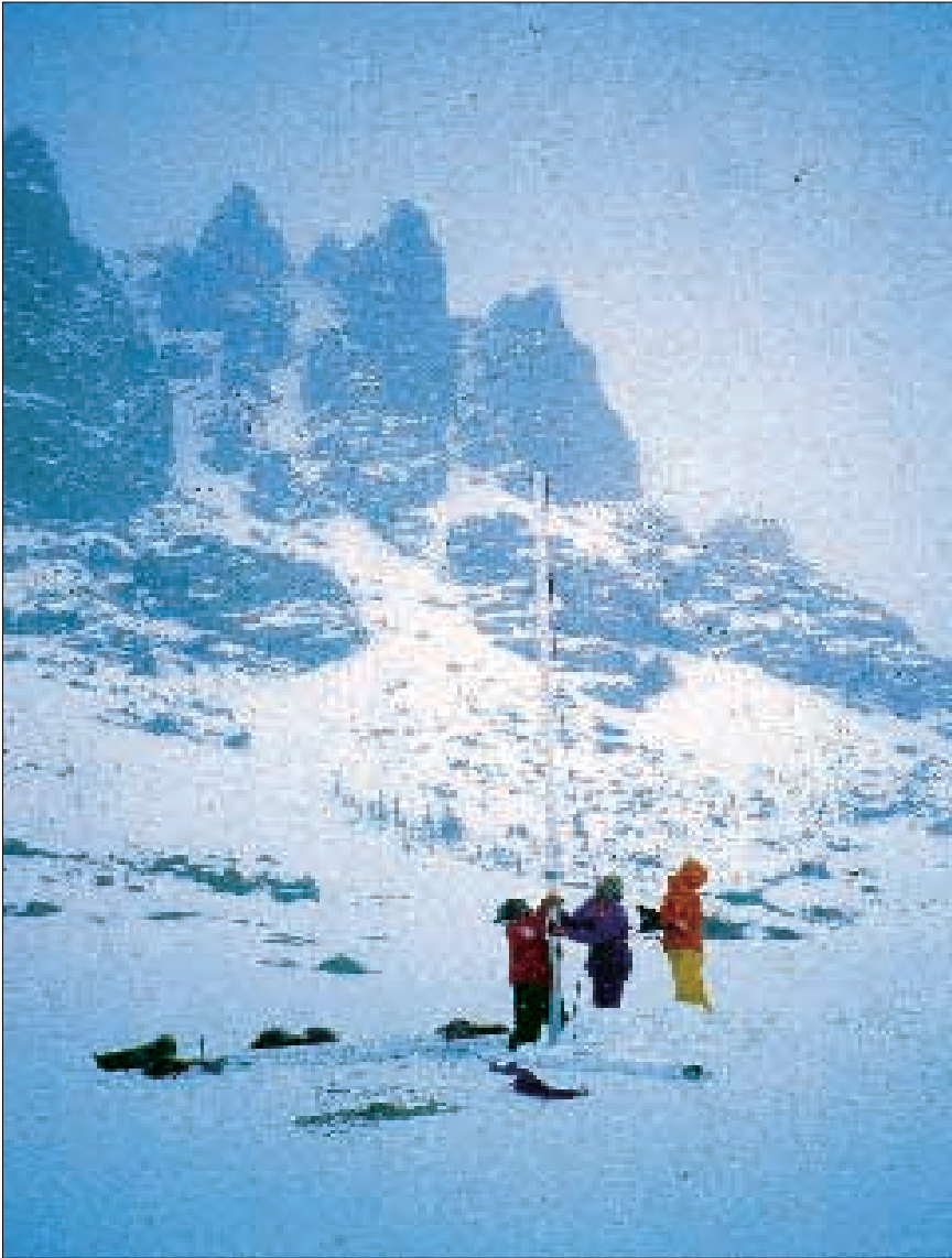
Fig. 2: A lightweight percussion coring system designed for remote access being used to recover a continuous 14,000-year lake sediment record from Sky Pond (3320 m asl) in the Colorado Front Range. The Sky Pond record provides the first clear indication that changes in late-glacial and early Holocene vegetation near timberline in the Rocky Mountains were in phase with the Younger Dryas climatic oscillation in the North Atlantic region. Additional paleo records from climatically sensitive high elevation sites are required from mountain regions around the world to complete the picture of regional paleoenvironmental changes.
